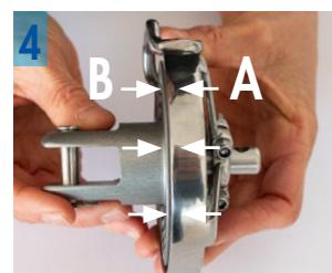
1-2. Pre-tighten the guide with the screws and nuts
