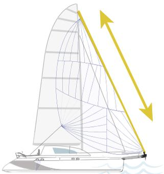
**2** Slightly tighten the sheet, then press the wireless remote control - or wired control button to furl in
