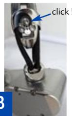
**Bottom :** connect the sail by engaging the pin until it locks. To disconnect, press the trigger to extract the pin.
