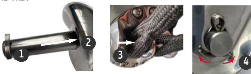
**4500 VERSION (Pin/screw)** : Engage the bridle axis (1) in the bridle attachment (2) by connecting it with the eye of the stropes, (3). Then screw in the 2nd screw with blue threadlocker (4) making sure that it fits into the countersink (5).
