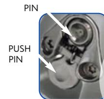
**Top :** open the trigger pin and connect the top of the sail. Then fit the protection cover
