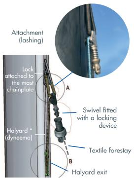
$^*$  Halyard partially without outer shell on 1.1 to 1.2 x the luff length
